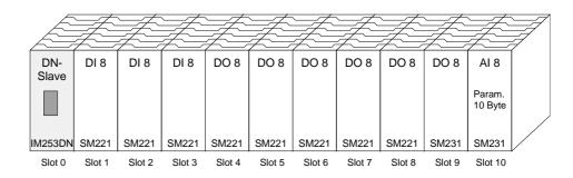
The example shows a DeviceNet coupler with 10 modules; however, the modules installed in plug-in locations 1 to 9 can not be configured.
